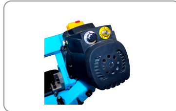
Speed controller, reset button, power on indicator
