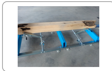
Log holding system
