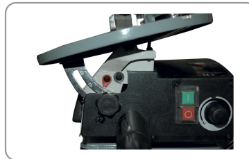
Cast aluminium table tilting at 45°
