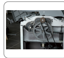
Rollers driven by chain, double-belt motor drive
