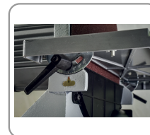
Cast iron table tilting at 45°
