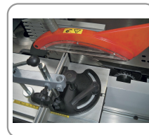
2000 mm sliding carriage flush with the blade, blade Ø 315 or 250 mm, scoring blade Ø 100 mm
