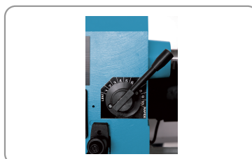
10 variable speeds from 500 to 2000 rpm
