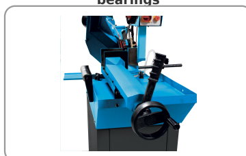
Quick clamping vice with slack adjustment lever
