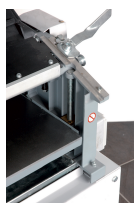
Cast iron thicknessing table mounted on 4 threaded rods
