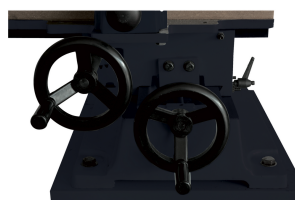
Lateral and longitudinal strokes on dovetail slides
