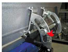
Profiled aluminium guide tilting at 45°
