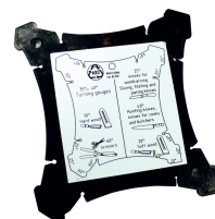
Angle measurement jig
