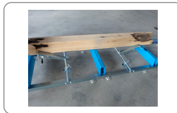
Log holding system
