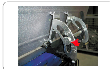
Profiled aluminium guide tilting at 45°
