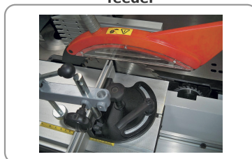
2000 mm sliding carriage flush with the blade, blade Ø 315 or 250 mm, scoring blade Ø 100 mm
