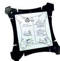
Angle measurement jig
